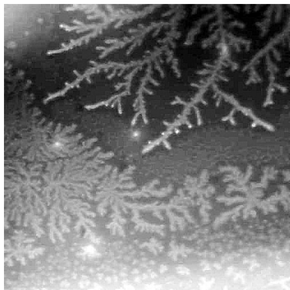
FIG. 2. 135 \times 135 \mu\text{m}^2 fluorescent image of two patterns of KCl crystals with different fractal dimensions grown in the presence of FITC-BSA with the fast drying method. Brightness is proportional to the concentration of FITC-BSA. The comparison with phase contrast and bright field images proves that albumin covers the crystals.
