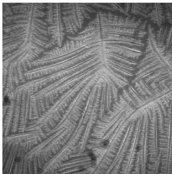
FIG. 4. 135 \times 135 \mu\text{m}^2 fluorescent image of stable tipped dendritic KCl crystals induced by a high concentration of albumin.
