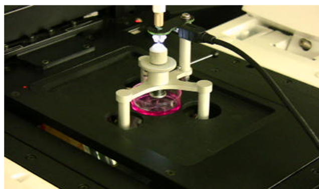
Figure 2 | Cell sorter micropipette in action. Video shows the micropipette when picking up 40 cells from a 35 mm Petri dish held by the motorized microscope stage. Pick up process of single cells is accompanied by the tapping sound of the liquid valve as it opens for 8 ms.
